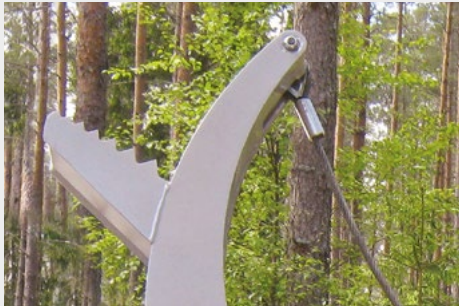
Stammablage an Klemmarmen trunk carrier at the clamping arms
